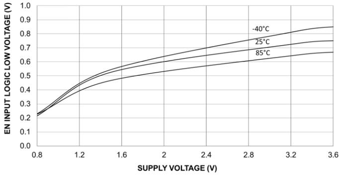
Figure 40. EN Input Logic Low Threshold
