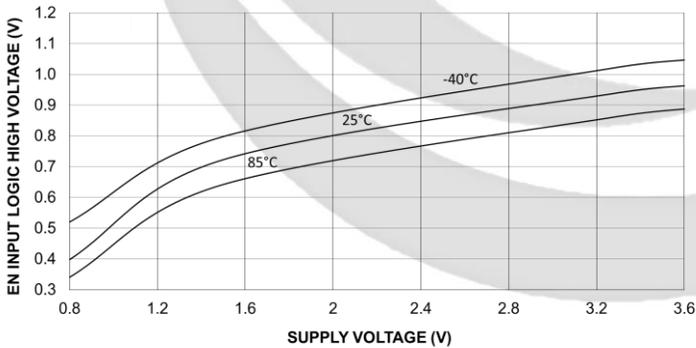
Figure 8. EN Input Logic High Threshold
