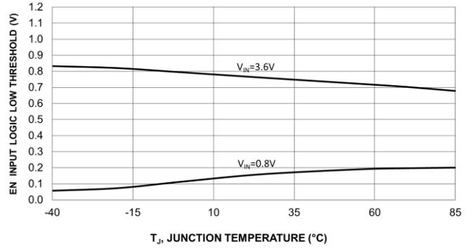
Figure 51. EN Input Logic Low Threshold Vs. Temperature
