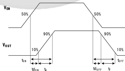
Figure 3. Timing Diagram
