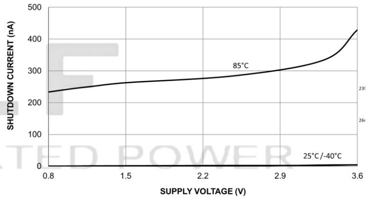
Figure 7. Shutdown Current vs. Supply Voltage
