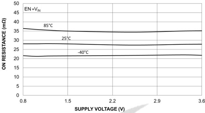
Figure 1. On-Resistance vs. Supply Voltage
