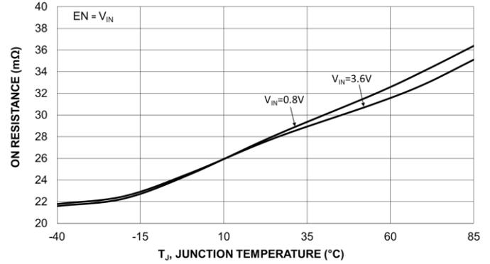
Figure 2. On-Resistance vs. Temperature
