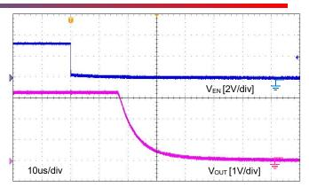
Figure 23. Turn-Off Response, GLF72101  $V_{\text{IN}}\text{=}3.3 \text{ V}, \text{ } C_{\text{IN}}\text{=}0.1 \text{ } \mu\text{F}, \text{ } C_{\text{OUT}}\text{=}0.1 \text{ } \mu\text{F}, \text{ } \text{R}_{\text{L}}\text{=}150 \text{ } \Omega$
