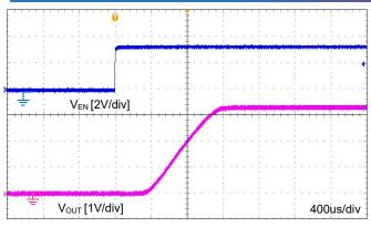
Figure 22. Turn-On Response, GLF72101 V\_{IN}=3.3 V, C\_{IN}=0.1 \ \mu\text{F}, C\_{OUT}=0.1 \ \mu\text{F}, R\_L=150 \ \Omega
