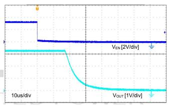
Figure 25. Turn-Off Response, GLF72103  $V_{IN}$ =3.3 V, C<sub>IN</sub>=0.1 µF, C<sub>OUT</sub>=0.1 µF, R<sub>L</sub>=150  $\Omega$
