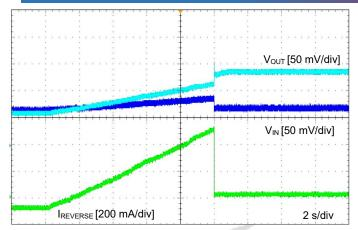
Figure 28. Reverse Current Blocking Threshold VIN=3.3 V, VOUT=Up to 3.4 V in CIN=0.1  $\mu F,$  COUT=0.1  $\mu F$
