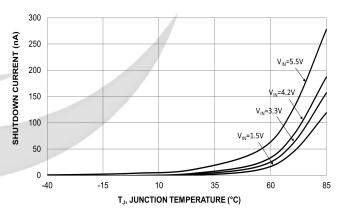
Figure 9. Shutdown Current vs. Temperature
