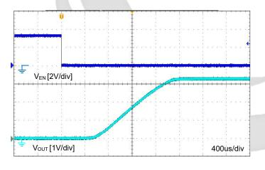
Figure 26. Turn-On Response, GLF72105  $V_{\text{IN}}{=}3.3$  V,  $C_{\text{IN}}{=}0.1$   $\mu\text{F},$   $C_{\text{OUT}}{=}0.1$   $\mu\text{F},$   $R_{\text{L}}{=}150$   $\Omega$
