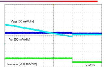
Figure 29. Reverse Current Blocking Release VIN=3.3 V, VOUT=Down to 3.2 V in CIN=0.1  $\mu F,$  COUT=0.1  $\mu F$
