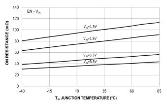
Figure 5. On-Resistance vs. Temperature
