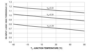
Figure 10. EN Input Logic High Threshold
