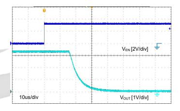
Figure 27. Turn-Off Response, GLF72105 V\_{IN}=3.3 V, C\_{IN}=0.1 \ \mu\text{F}, C\_{OUT}=0.1 \ \mu\text{F}, R\_L=150 \ \Omega
