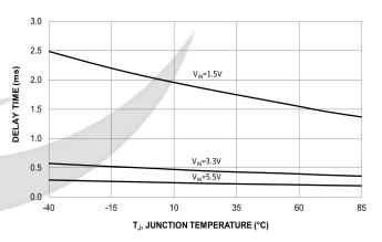
Figure 15. Turn-On Delay Time vs. Temperature GLF72100 and GLF72101
