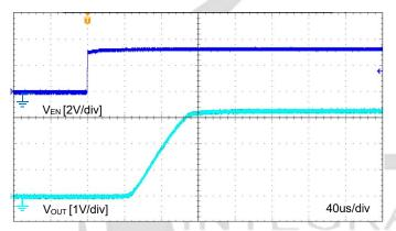
Figure 24. Turn-On Response, GLF72103 V<sub>IN</sub>=3.3 V, C<sub>IN</sub>=0.1 μF, C<sub>OUT</sub>=0.1 μF, R<sub>L</sub>=150 Ω
