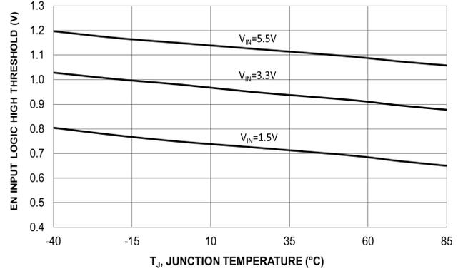
Figure 11. EN Input Logic High Threshold Vs. Temperature
