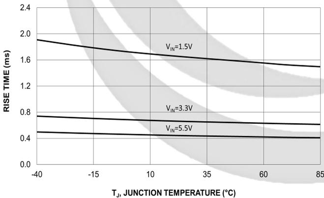
Figure 14. V<sub>OUT</sub> Rise Time vs. Temperature
