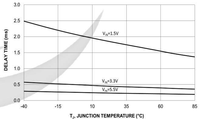
Figure 15. Turn-On Delay Time vs. Temperature
