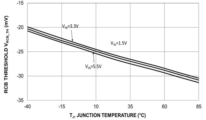
Figure 17. RCB Threshold Voltage vs. Temperature
