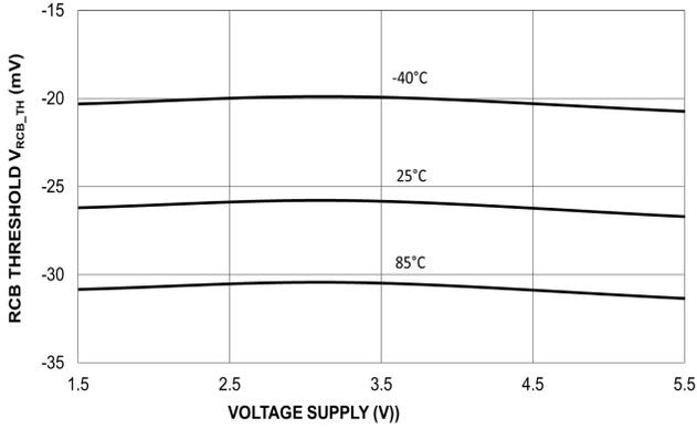
Figure 16. RCB Threshold Voltage vs. Supply Voltage
