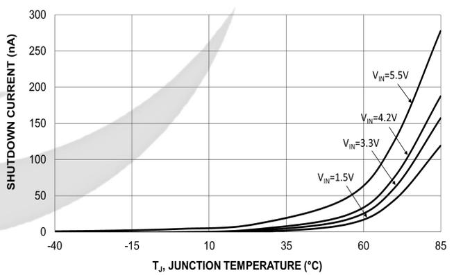
**Figure 9. Shutdown Current vs. Temperature**
