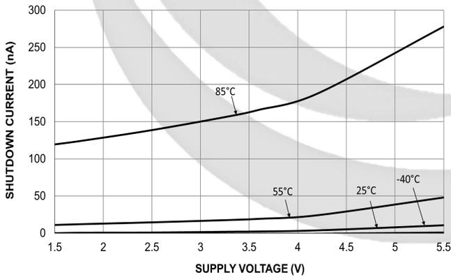
**Figure 8. Shutdown Current vs. Supply Voltage**
