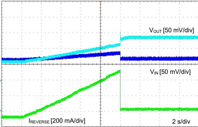
**Figure 28. Reverse Current Blocking Threshold**
