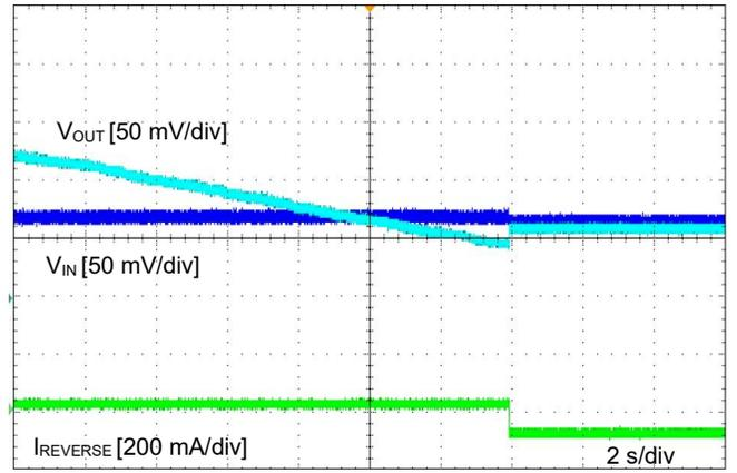
**Figure 29. Reverse Current Blocking Release**
